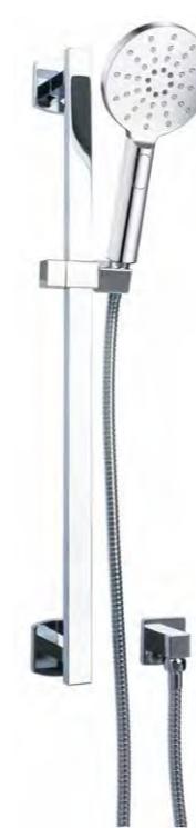
FWM9539M with 3 spray functions Slide shower 600mm centres WELS 4 star 6.5L/min
