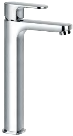
FWS9889B Tall basin mixer 260mm aerator height x 120mm reach, chrome WELS 5 star 5L/min
