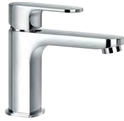
FWS9889 Standard basin mixer 100mm aerator height x 120mm reach, chrome WELS 5 star 5L/min
