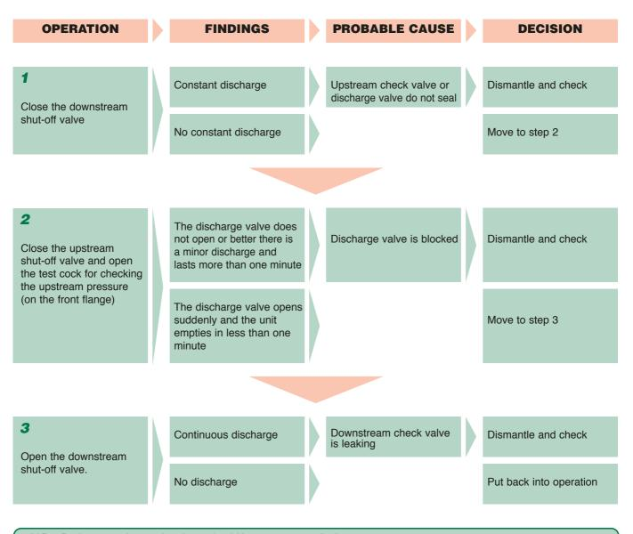
N.B. : During normal operation there should be no constant discharge. If there is a constant discharge dismantle and inspect the device.
