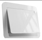
The IB215 requires an opening of  $275 \times 210$ mm. It has four bendable tabs which fold over the dry wall lining and hold the plate securely without drilling or screwing. The hinged lid is easily removed from the frame by opening and pushing reward the lid to disengage the hinge. The lid and frame are powder coated steel and suitable for indoor application only.
