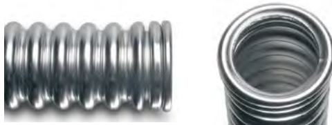
Poorly compressed corrugations
