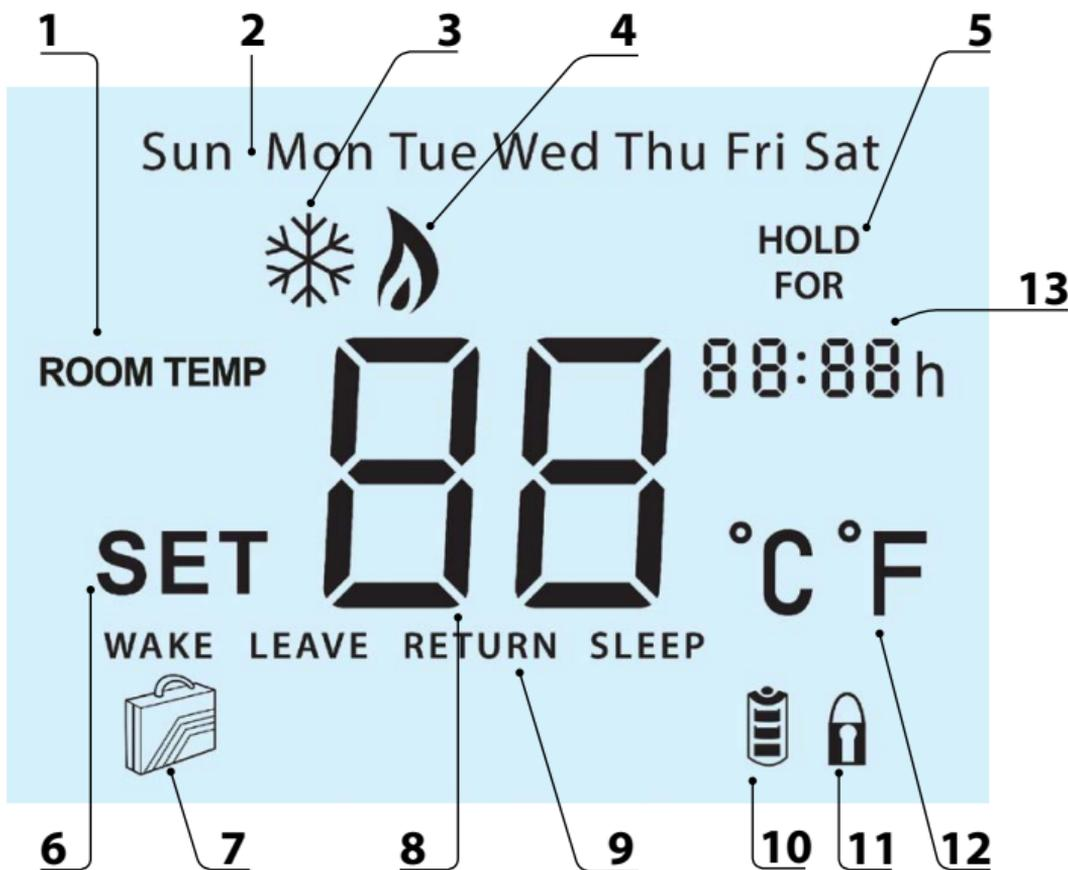
1. Room Temp - Indicates the current temperature sensor mode.
