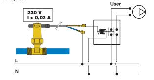
**N.B.:** It is recommended to pay attention to the current consumption value of the user device the flow switch is connected to. If this value is greater than **0,02 A**, a relay must be installed between the flow switch and the user device itself to prevent damage to the flow switch contacts.
