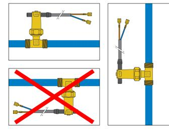
The 315 series flow switch can be installed on either vertical or horizontal piping, but not upside down. The top part of the flow
