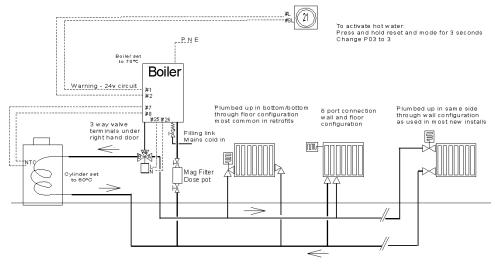
System output up to 25kW 20mm pipe System output up to 45kW 25mm pipe
