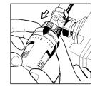
**3.** Re-lock the ring. The valve will now be locked at the set temperature.
