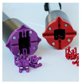
Make sure that the colour of the fixation is the same as the colour of the clip.
