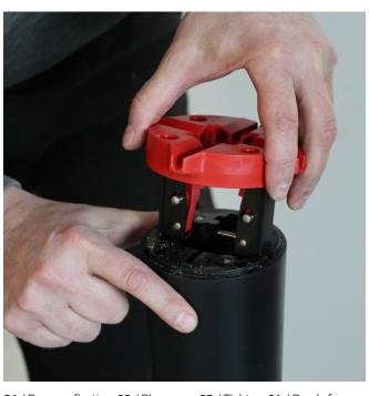
$\bf 01$  / Remove fixating.  $\bf 02$  / Place new.  $\bf 03$  / Tighten.  $\bf 04$  / Ready for use
