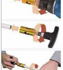
cut pipe in order to prevent unintentional o-ring damage as the pipe is inserted. For the same reason it is good practise to use Vinoleo or Greasil lubricant on all sizes and essential on fittings 26mm and bigger.
