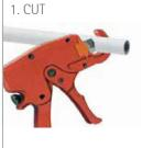
The pipe must be cut square. Good quality shear style cutters can be used on 16 and 20mm sizes. Rotary style cutters should be used on bigger sizes to prevent squashing and distortion.
