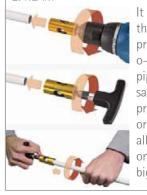
It is <u>critical</u> to ream the cut pipe in order to prevent unintentional o-ring damage as the pipe is inserted. For the same reason it is good practise to use Vinoleo or Greasil lubricant on all sizes and essential on fittings 26mm and bigger.
