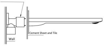
The inwall G1/2" female thread must be recessed or not exceed the cement sheet as shown.
