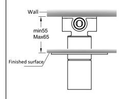
Total adjustment range measured from wall to finished surface is 55mm to 65mm.
