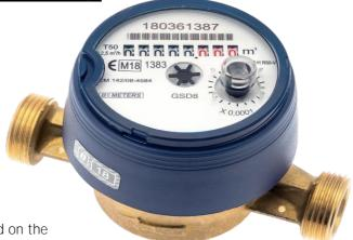
The meter can be installed according to what is indicated on the dial H: horizontal water flow V: vertical water flow  $\uparrow$ = dial on top  $\rightarrow$ = dial on the side
