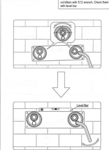
Adjust two eccentric connectors to level
