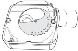
Fig. 23 - 50/70 burner air adjuster disc (shown set to position 'C')
