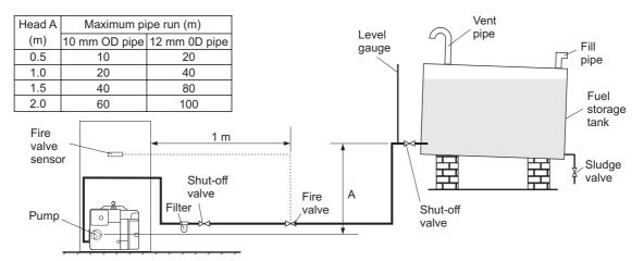
Fig. 2 - Single pipe system
