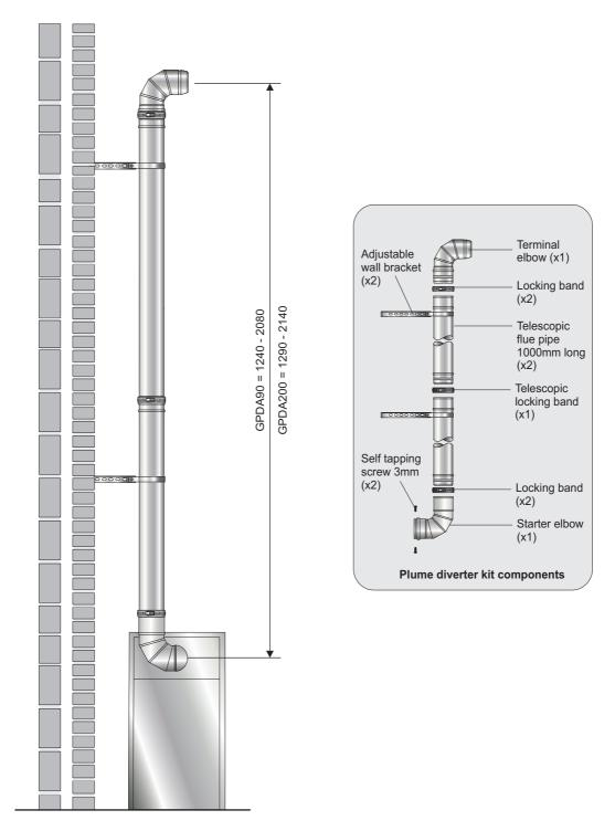
Fig. 16 - Plume diverter kit (Outdoor boiler)
