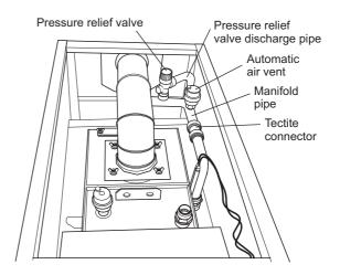
Fig. 18 - 50/70 top view (showing automatic air vent, pressure relief valve and manifold)
