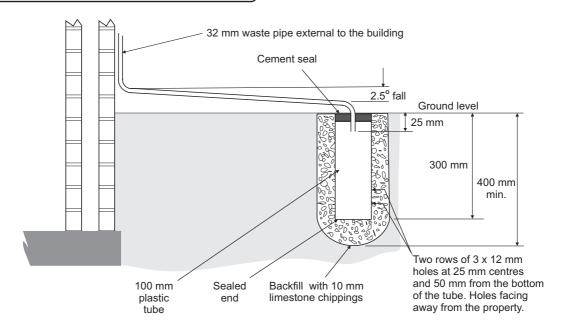
Fig. 13 - Purpose made condensate soakaway
