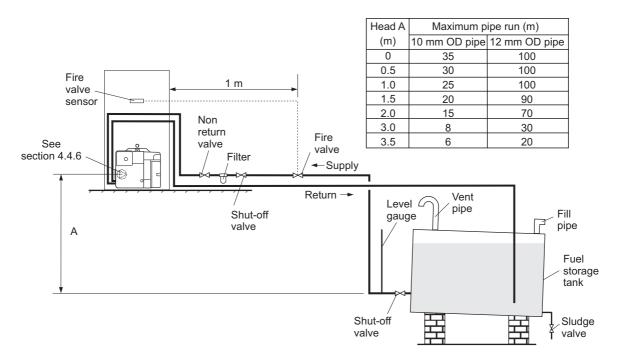
Fig. 3 - Two pipe system
