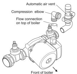
Fig. 20 - Sealed system pump assembly
