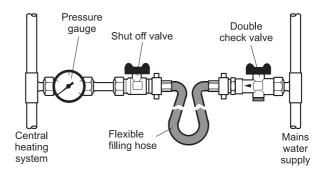
Sealed system filling loop arrangement - Fig. B
