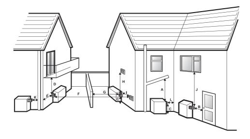
Fig. 7 - Clearances for flue terminals
