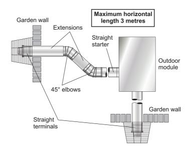
Fig. 17 - Horizontal external flue
