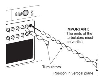
Fig. 28 - Removal/replacement of spiral turbulators (50/90 shown)
