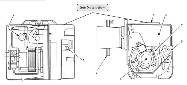
Fig. 21 - RDB burner components
