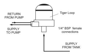
Fig. 5 - Tiger loop 'de-aeration' device
