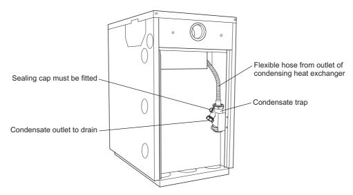
Fig. 11 - All models rear view (panel removed)
