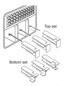
Fig. 26 - 90/120 and 120/155 baffles
