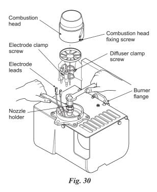
3 Check the electrode and diffuser settings - Fig. 31
