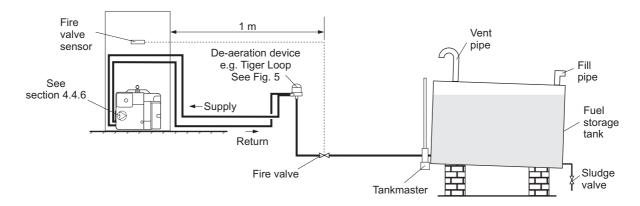
Fig. 4 - De-aeration device system
