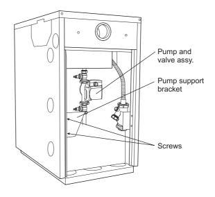
Fig. 19 - 50/70 rear view (showing pump assembly)
