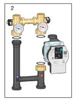
Position the connecting pipe on the right-hand side, rotating it on its axis by 180°.
