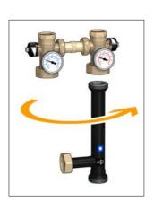
In versions with UPML 25-95 pump, it is necessary to rotate the electronic part of the pump, unscrewing the four screws, as indicated by the arrows, and turning the body anticlockwise by 90°. If this step is not performed, it will not be possible to fit the unit back inside the insulation.
