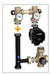
3. Unscrew the cap on the right-hand side of the mixing valve and screw it onto the opposite side.
