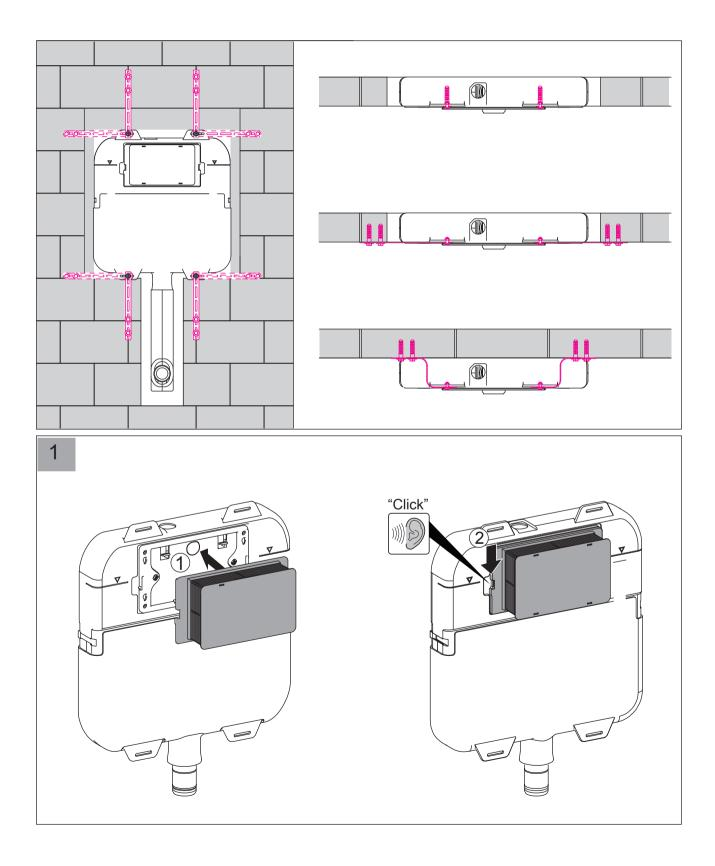
FRONT OF WALL CISTERN INSTALLATION (e.g. when installing in front of a brick wall)
