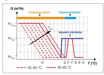
The graph shows the variation of the Kv value depending on the device configuration (A, B, C) and on the inlet temperature of the domestic hot water.
