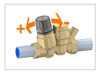
The graduated scale shows the temperatures at which the indicator can be set. It is recommended to set the valve temperature at a value about 5K greater than the water temperature at the valve inlet, taking into account the heat losses along the line, to limit the head required at the recirculation pump. Take care to ensure the minimum flow rate at the mixing valves in the central heating system.
