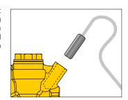
This system allows disinfection control in each circuit and optimization of the disinfection process. In this case it is possible to measure and monitor the water temperature in each circuit, even from remote.
