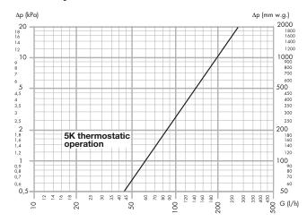
To choose the recirculation pump head, the head loss at the valve should be added to the head loss in most disadvantaged circuit.
