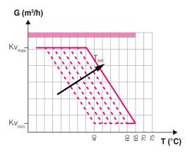
The graph shows the variation of the Kv value depending on the device configuration and on the inlet temperature of the domestic water.
