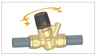
The graduated scale shows the temperatures at which the indicator can be set. It is recommended to set the valve temperature at a value about 5K greater than the water temperature at the valve inlet, taking into account the heat losses along the line, to limit the head required at the recirculation pump. Take care to ensure the minimum flow rate at the mixing valves in the central heating system.
