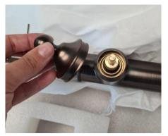
2. Undo the finishing cap, and undo the grub screw located on the underside of the brass stem – remove stem from cartridge (photo 3)
