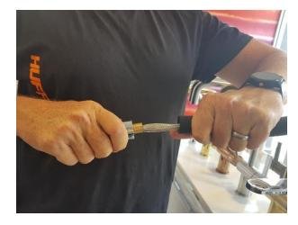
2. Get a firm grip on the flexi hose; hold it as close to the brass as possible and twist the handpiece.
