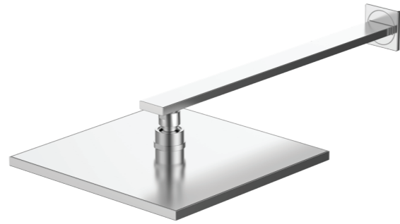
FWCU09BN Wall mounted rain shower brushed nickel Recommended working pressure 200 - 500kPa (balanced) WELS 8 star 9L/min
