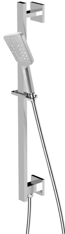
FWCU9507BN 600mm centers and 15mm integrated connection, brushed nickel 1500mm metal wound shower hose Recommended working pressure 200 - 500kPa (balanced) WELS 4 Star 6L/min
