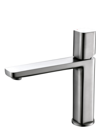
FWCU8228BN Standard basin mixer brushed nickel 122mm aerator height x 148mm reach Recommended working pressure 200 - 500kPa (balanced) WELS 4 Star 6L/min
