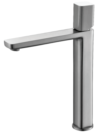
FWCU8268BN Tall basin mixer brushed nickel 234mm aerator height x 172mm reach Recommended working pressure 200 - 500kPa (balanced) WELS 4 Star 6L/min
